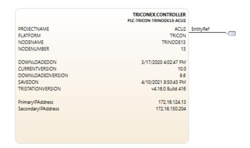
Control Modules that represent PLC Program Logic are named using the format: PLC-NodeName-LP-ProgramName where NodeName is the name of the PLC node extracted from the "Project Implementation" document and the ProgramName is the name of the Logic Program. i.e. PLC-TRICON1-LP-COMPRSD.
