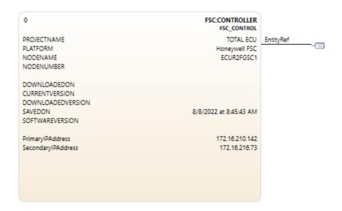
Control Modules that represent FSC PLC Program Logic are named using the format: *NodeName* where *NodeName* is the name of the FSC Controller node.
