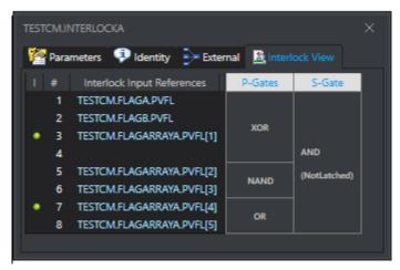
The Interlock View tab item when selected in the Properties View will present a visualization of its configured gate logic. The LED status item in the first column represents the inversion status of the input.
