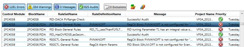
The Results view contains the messages emitted by the rules when executing policy validation. You can copy and paste these results into Excel using **Ctrl+C/Ctrl+V** keys. You can navigate to the Control Module Chart View by left mouse double-clicking on a result item.
