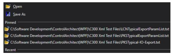
Right mouse-click on an MRU path item to view its context menu that allows you to remove the item or toggle its pinned state.
